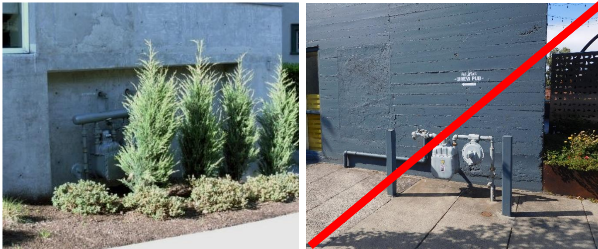
Figure 2.5.B Acceptable and unacceptable utility meter location and screening examples.
